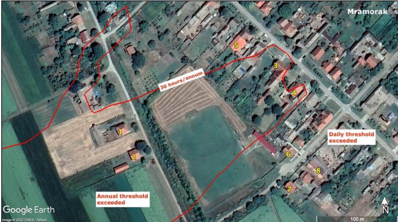
Figure 12-3 Receptors Predicted to be Affected by Shadow Flicker in Mramorak Village (aerial image date: 25 October 2021)
