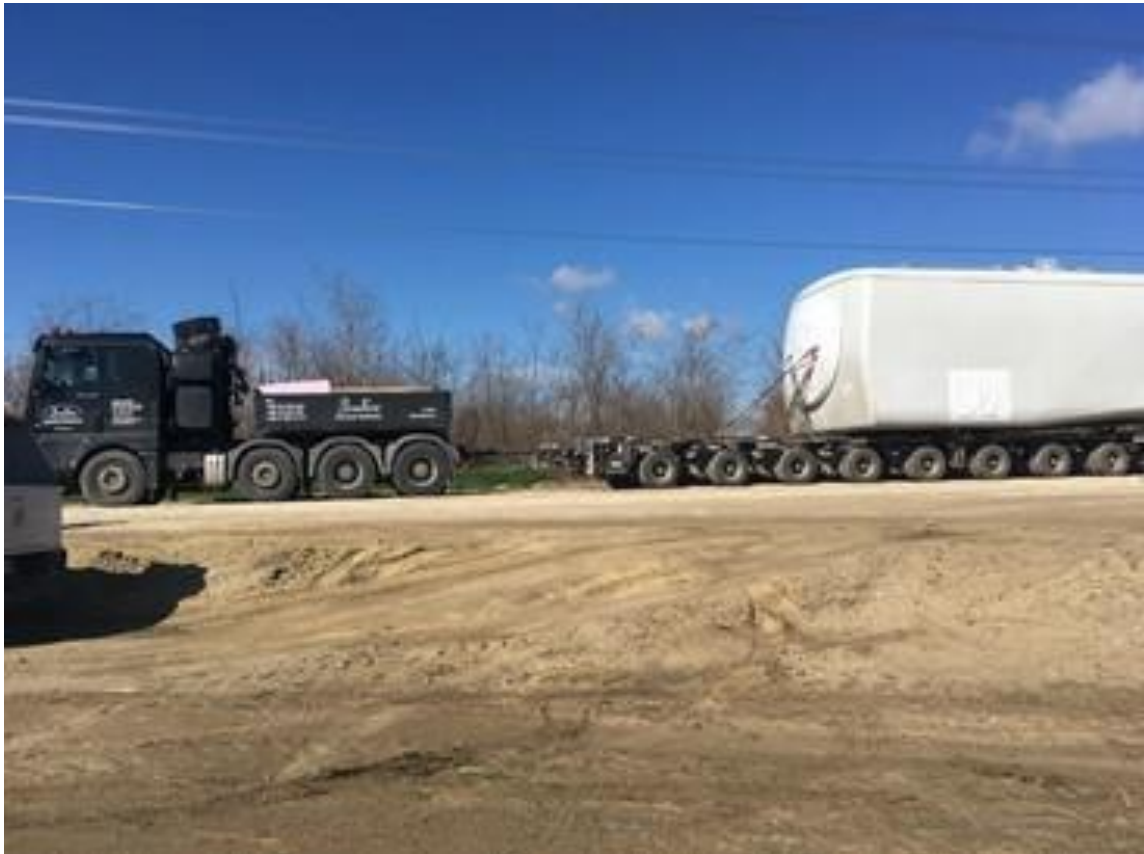
Figure 5-17 Delivery of a WTG nacelle
